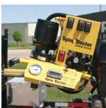
The tilting head allows for easily attaching to valves that aren't aligned perfectly vertical.
