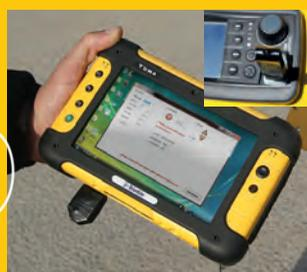
Data is transmitted to a field computer, or stored in the on-board computer and transferred to flash drive.
