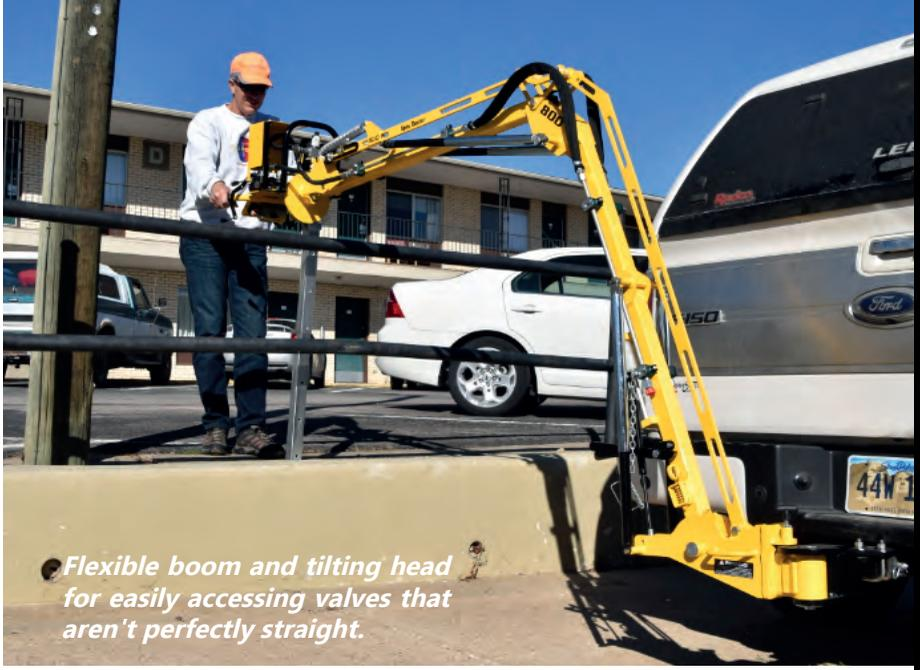
Flexible boom and tilting head for easily accessing valves that aren't perfectly straight.
