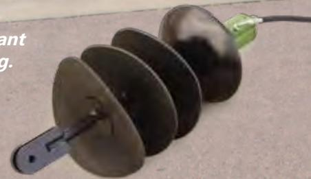
*Re-rounder for repairing deflected pipelines*
