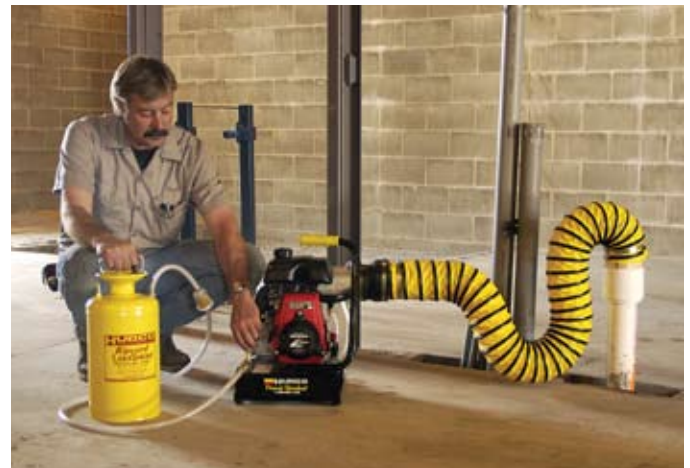
Typical set up for Smoke Testing
